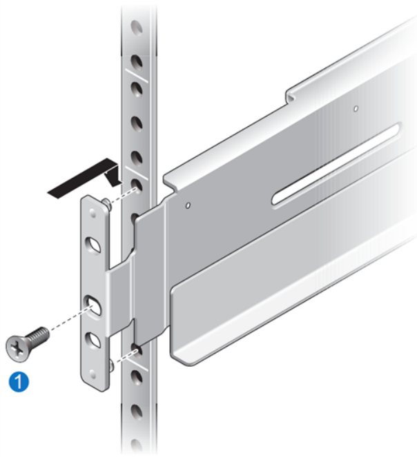
Figure 13: Attaching front rail assembly
