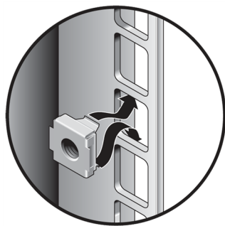
Figure 12: Cage nut installation
